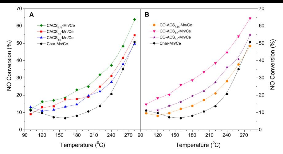
NO conversion (%) of chemically activated (CACS<sub>x</sub>-Mn/Ce) and co-activated (CO-ACS<sub>x</sub>-Mn/Ce) cotton stalk derived SCR-deNO<sub>x</sub> catalysts impregnated with Mn/Ce. A = CACS<sub>x</sub>-Mn/Ce, B= CO-ACS<sub>x</sub>-Mn/Ce.
