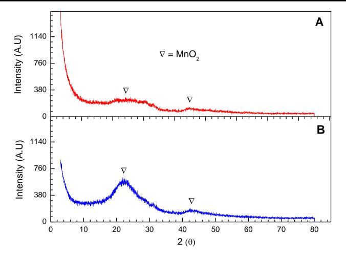
X-ray diffraction patterns of chemically activated (CACS<sub>x</sub>-Mn/Ce) and co-activated (CO-ACS<sub>x</sub>-Mn/Ce) cotton stalk derived SCR-deNO<sub>x</sub> catalysts impregnated with Mn/Ce. A = CACS<sub>1.5</sub>-Mn/Ce, B = CO-ACS<sub>1.5</sub>-Mn/Ce.
